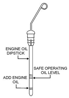
Figure 7. Engine Oil Dipstick
